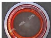
Copper tube butt welding
